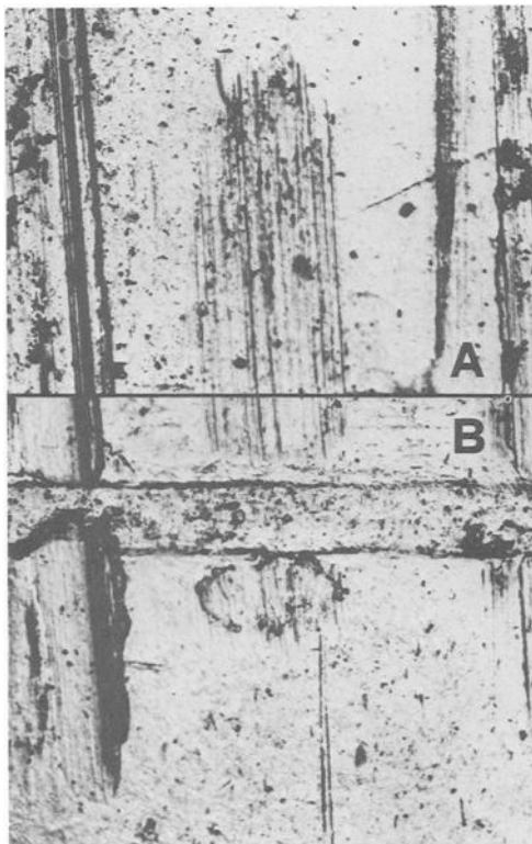
FIG. 3—The correspondence between marks in close-ups of replicas obtained from the lateral surface of two different bullets (a) and (b) fired by the same weapon (semiautomatic Beretta pistol Model 34, 7.65 mm) (macrophotograph).
